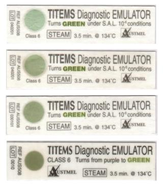
**PASS**: **GREEN IS GOOD!** Different sterilizers produce varied results depending on quality of steam, as long as the emulator has turned **GREEN** the parameters have been met.
